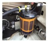
Utilization of the particle as well as filter technology offered by iCerMax™ may be seen in the use of the DUO-AquaTrap™, which is considered a market leader in addressing both free water as well as suspended water and particulate contamination. The unique pre-filter was developed in Africa so as to endure the harshness of the unique African conditions. The system incorporates a 3
